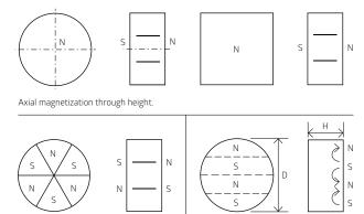
Sector shaped magnetization axially magnetized through height.
