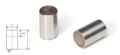
The holding force will be reduced up to 15 percent due to magnetic short circuits when the magnetic system is directly installed in iron. In order to prevent this, certain distances must be observed from the brass housing of the magnetic system to the iron. The distances to the iron shall also be observed when the magnetic system was shortened by the dimension KM. Please see the recommended distances from the table (distance mm).
