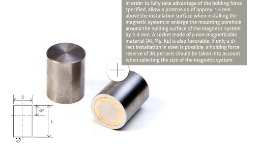
Magnetic system cylindrical, with fitting tolerance h6, magnetic core AlNiCo 500
