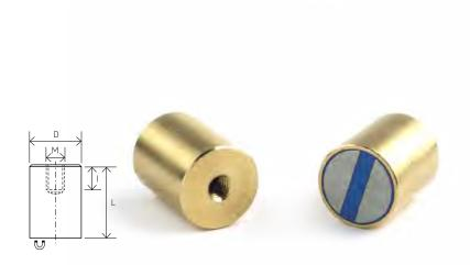
Magnetic system cylindrical, with fitting tolerance h6, with inner thread, magnetic core NdFeB
